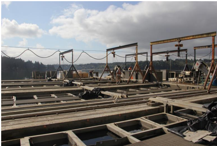
Figure 2. FLUPSY Subsystem Used in Oyster Aquaculture
