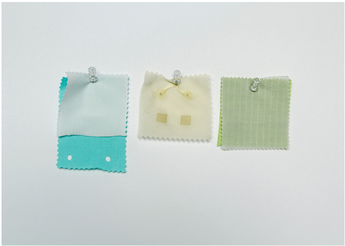
Figure 5.4. Material Variations. Layered and partially overlapped fabrics were explored as possible ways to introduce richer tactile behavior.
