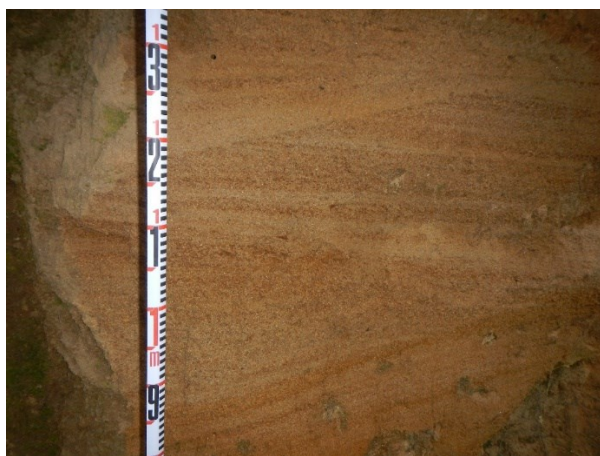
Figure B1. Close up photograph showing fluvial deposit from the modern Siang River with cross-bedding.
