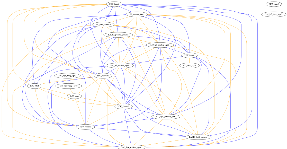
FIGURE 6.4: A snapshot of an undirected dependency graph display from a simulated run. Correlated components have been isolated, with edges drawn for all correlation relationships exceeding a certain value ( r_{PCC}^2 > 0.8 ). Both positive and negative correlation connections are shown. Self-correlations are not shown.
