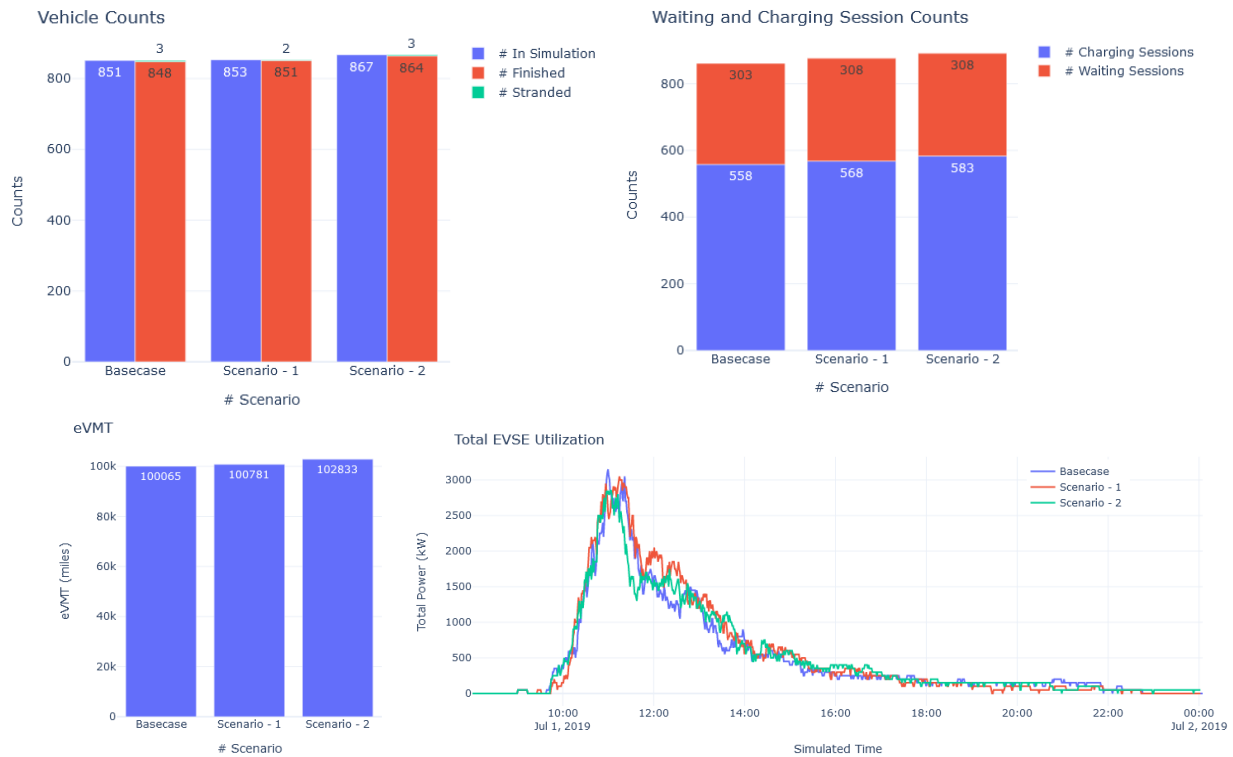
Figure 19: Comparison of EV counts (in simulation, finished and stranded) (top-left), charging session and waiting session counts (top-right), eVMT (bottom-left) and total EVSE utilization (bottom-right) for base-case, Scenario 1, and 2.
