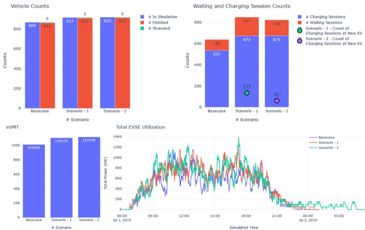
Figure 27: Comparison of EV counts (in simulation, finished and stranded), charging session and waiting session counts, eVMT and total EVSE utilization for base-case, Scenario 1, and Scenario - 2.
