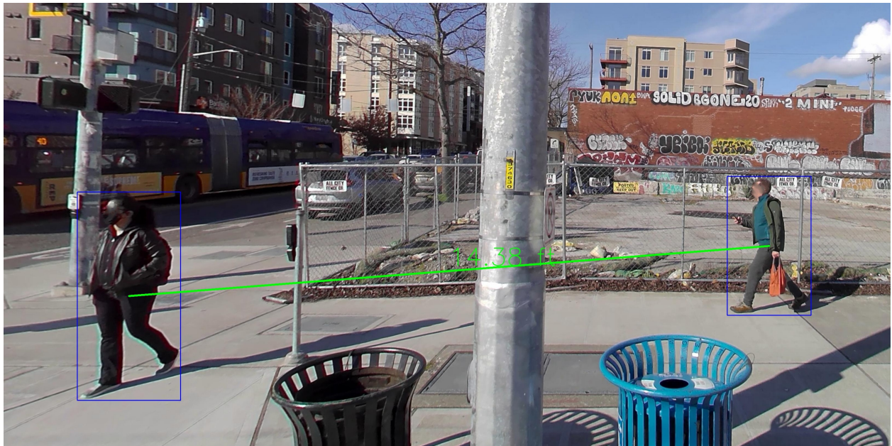
Figure 4.1: Sample output of the pedestrian detection and social distance estimation algorithm. There are 2 pedestrians, with an estimated 14.38 ft between them. Additional sample images are available in the supplementary material.
