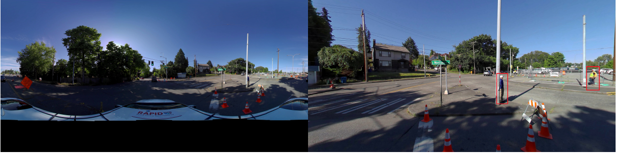
Figure 3.1: Sample images from the pedestrian detection data pipeline. The left image is an original 360° image from a data collection run. The image on the right is the right-hand side of the original image after orthorectification and pedestrian detection (both sides of the image are processed separately). There are two pedestrians that were detected by the algorithm (in red bounding boxes).
