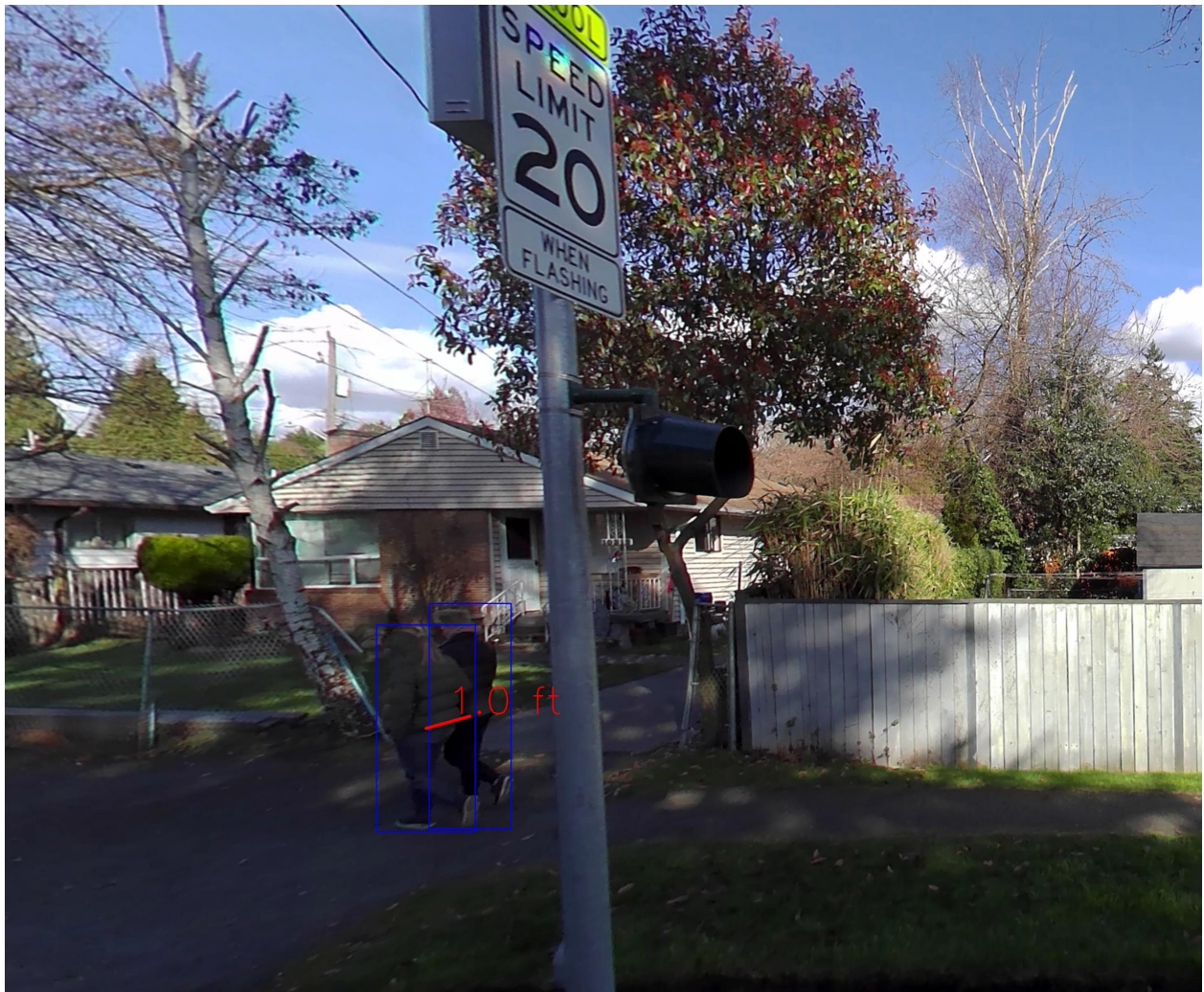
Figure A.3: Sample output of the pedestrian detection and physical distancing algorithm. This image contains two pedestrian walking nearby each other walking parallel with the vehicle.
