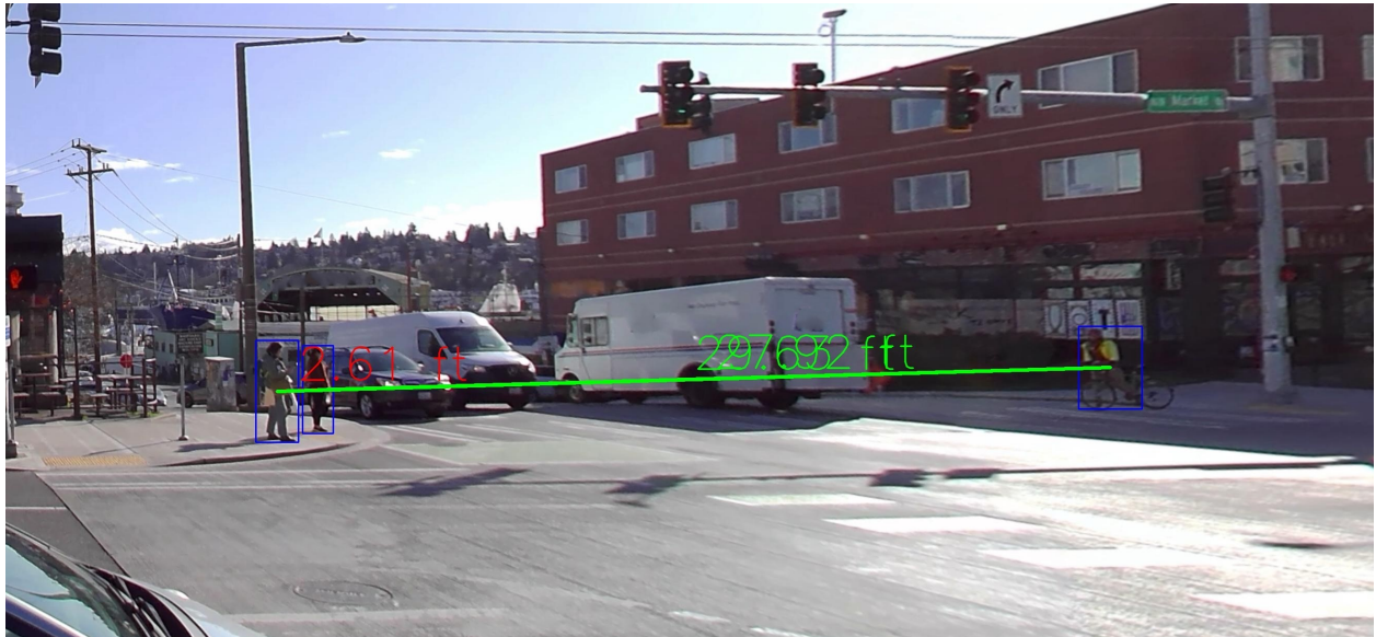
Figure A.1: Sample output of the pedestrian detection and physical distancing algorithm. This image contains two pedestrians near each other on one side of the street, about 30 feet away from a pedestrian across the street.
