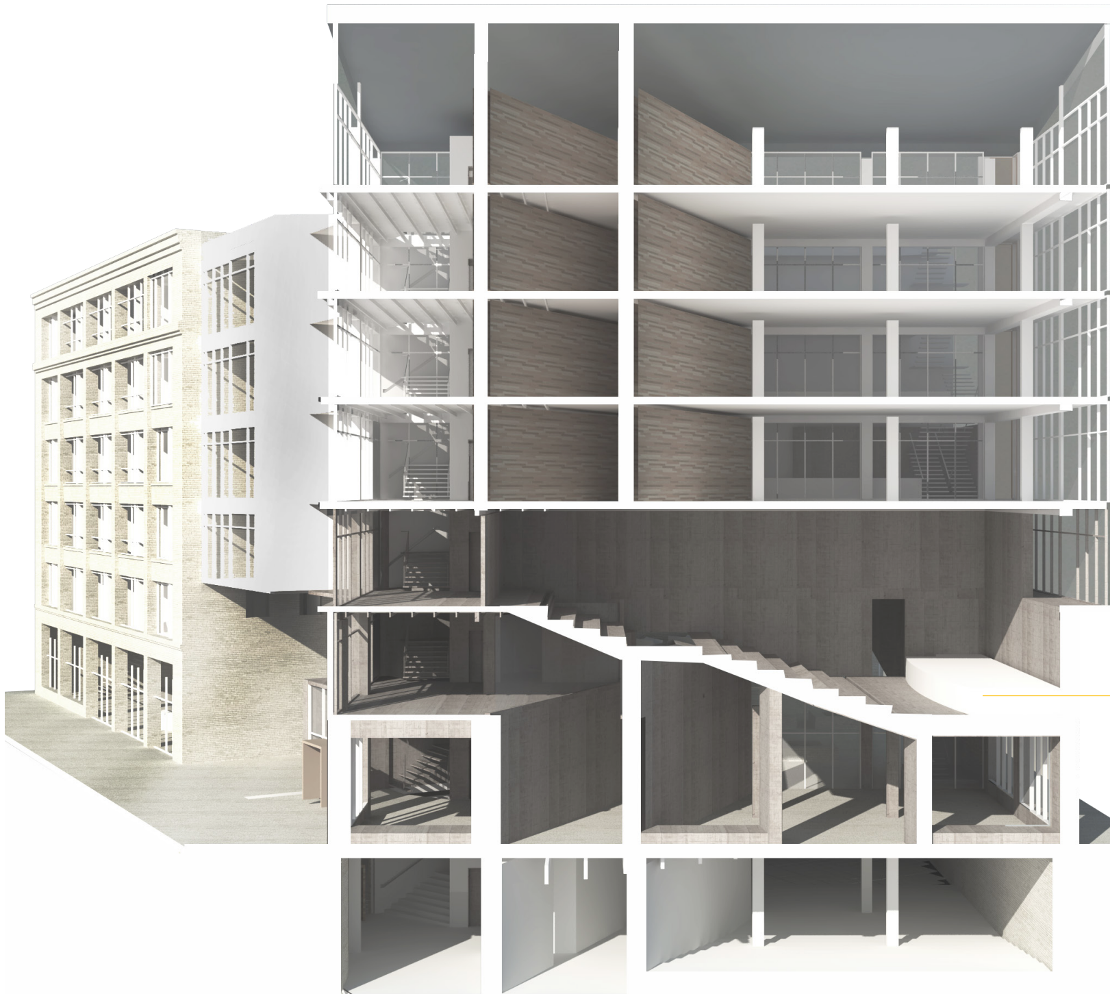
FIGURE 4.19 EAST WEST SECTION CUT THROUGH THE SOUTH BUILDING SHOWS THE STRUCTURE OF THE PERFORMING HALL AND THE PROSPECT AND REFUGE OPPORTUNITIES WITHIN.
