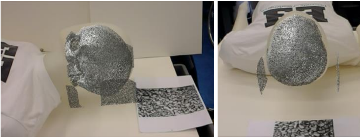
Figure 20: Image overlay using fiducial markers
