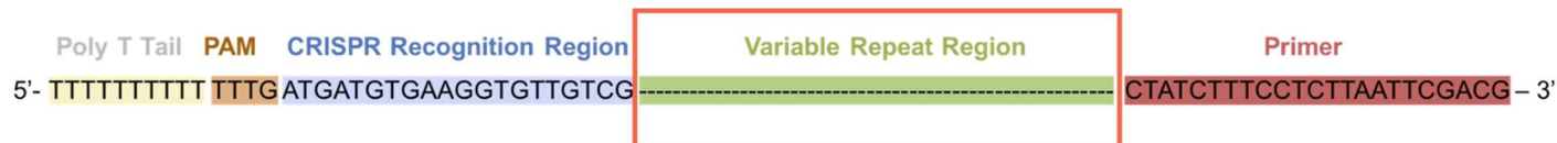
Figure 2. General structure of REACTR template strand, composed of poly T tail, PAM, CRISPR recognition region, variable repeat region, and primer. Variable repeat region is edited to account for drug specificity and then optimized.
