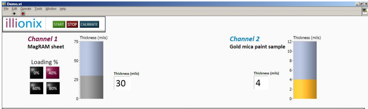
Figure 4-33. Screenshot of the in-process measurement program GUI.
