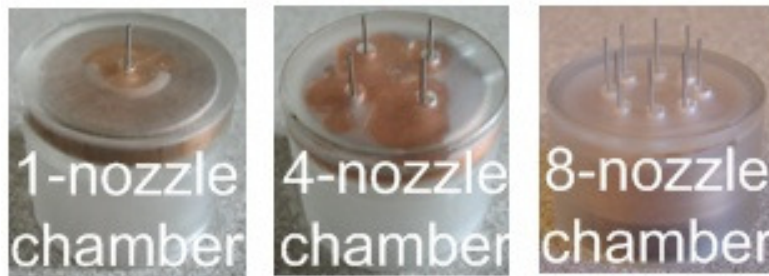
Figure 5-6. The assembled 1-nozzle chamber, 4-nozzle chamber (5 mm spacing), and 8-nozzle ESEC chamber (5 mm spacing).
