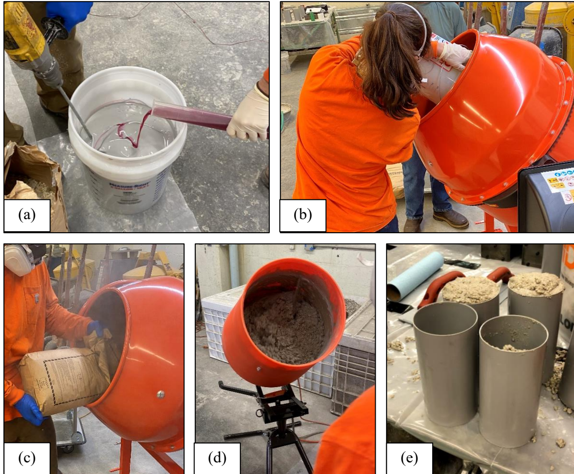
Figure 3-1. (a) Mixing of MEKP and HCSC resin with a squirrel cage mixer, (b) Resin mixture being transferred from mixing bucket to drum mixing, (c) Adding the pre-packaged aggregate and fiber blend to the drum mixer, (d) HCSC mix turning in drum mixer, (e) HCSC placed in cylinder molds before finishing
