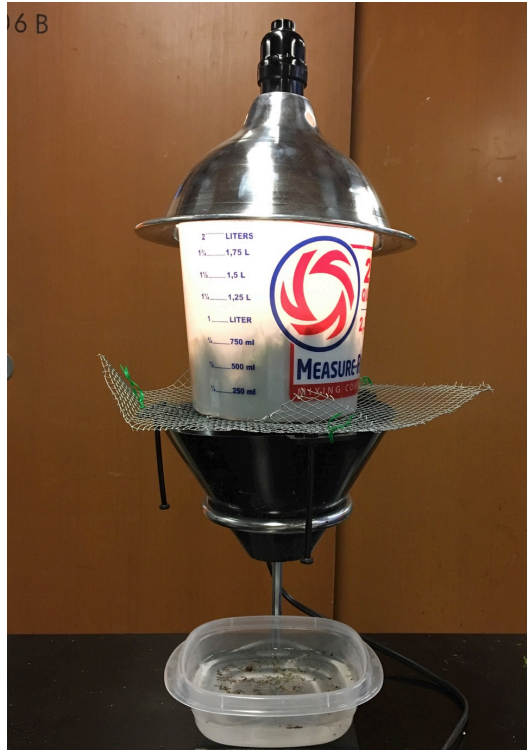
Figure 2.1 Tullgren funnel setup showing overhead view of moss (left) and frontal view of whole system extracting microarthropods out of the moss into DI water in a Tupperware® container
