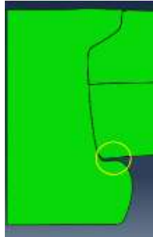
Figure 7.2. Axial Gap found in Percussive Simulation (circled in yellow).
