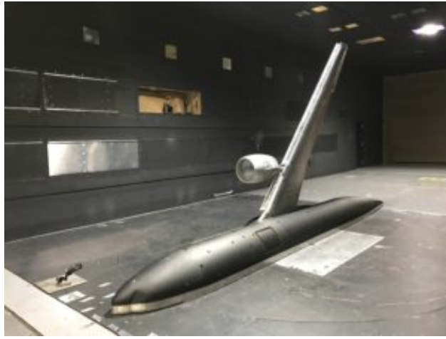
Figure 1.2: High Lift CRM installed in the 14x22 foot subsonic tunnel at NASA Langley Research Center [1]
