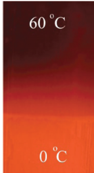
Figure 1.6: Response of a temperature-sensitive paint to a temperature gradient on a flat surface. The plate was heated and then one end was dipped in ice water. The dark end is hot and the bright (orange) end is cold 2
