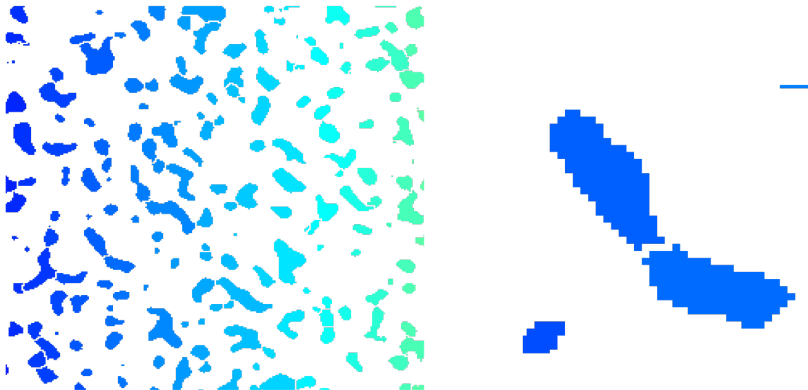
Figure 3.8. (Left) The segmented image is magnified so that individual grains and their predicted necks can be seen. (Right) An object from the segmented image with its predicted neck.
