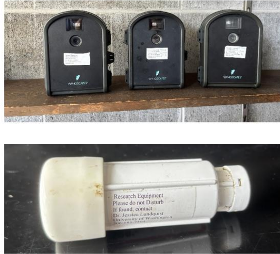
Figure 3: Field equipment – WingScape time lapse cameras and a HOBOWare TRH sensor.
