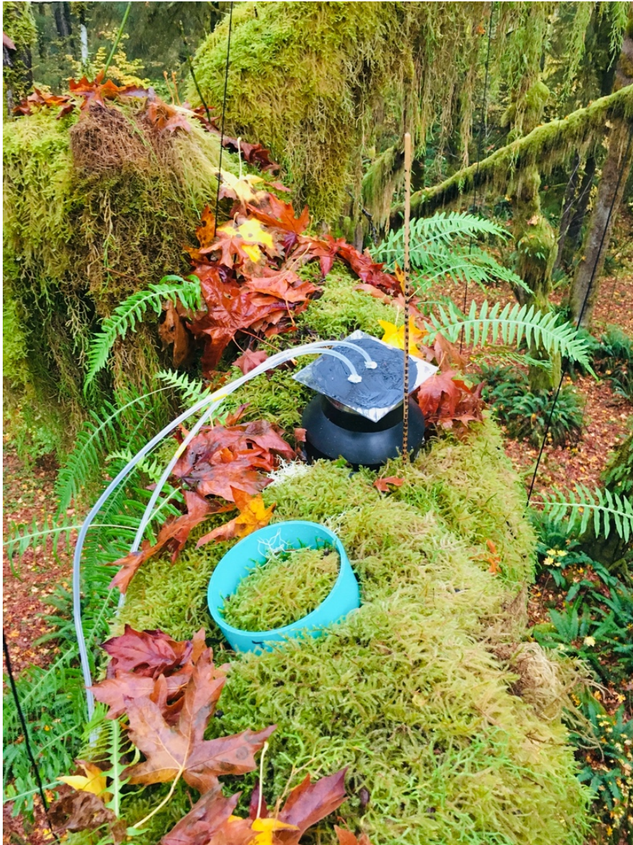
Figure 5. Canopy soil flux measurements conducted in a bigleaf maple tree in the Hoh Rainforest on the Olympic Peninsula of Washington state, USA. The black cap seals the top of a blue PVC collar placed in the canopy soil. Tubes from the cap transport gases from the enclosed soil chamber to the LGR greenhouse gas analyzer on the forest floor
