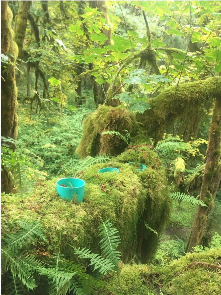
Figure 4. PVC collars were placed in canopy soil of bigleaf maple trees in the Hoh River Rainforest. Collars were placed at least 24 hours before measurements and remained through the 5-month duration of the study.
