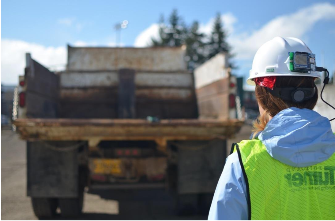
Figure 5.1 Worker-on-foot with device for monitoring location and orientation
