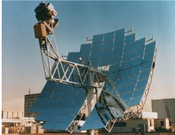
Figure 13 McDonnell Douglas Solar Stirling engine system [31]
