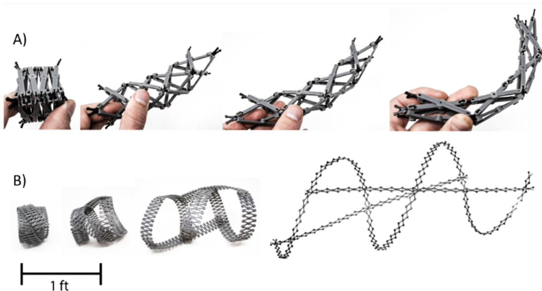
Figure A.4: Alternate HERDS and substructure variations. A) Adjusting link lengths creates bending deployment in triangular scissor mechanisms. B) HERDS can also be created from scissor mechanisms and Handed Shearing Auxetics (HSAs).
