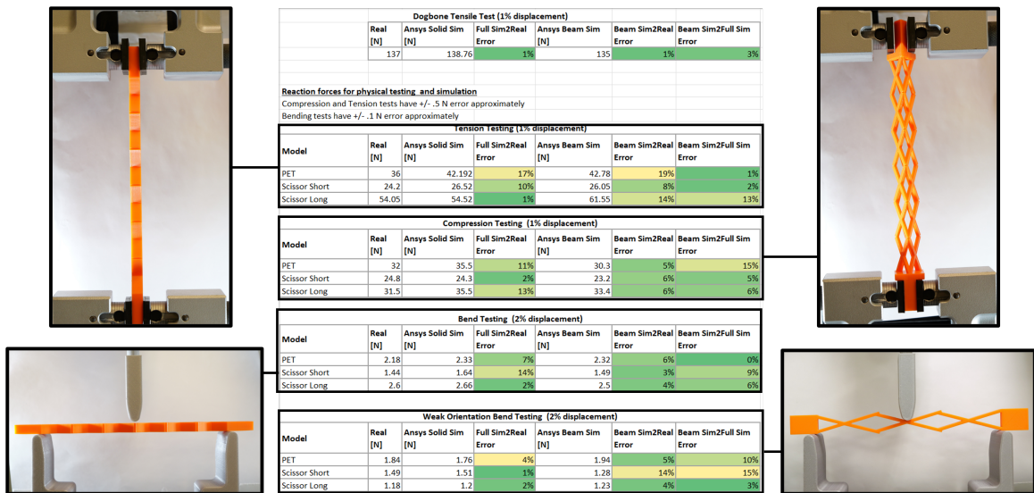
Figure A.7: We see close agreement between physical testing and simulation.
