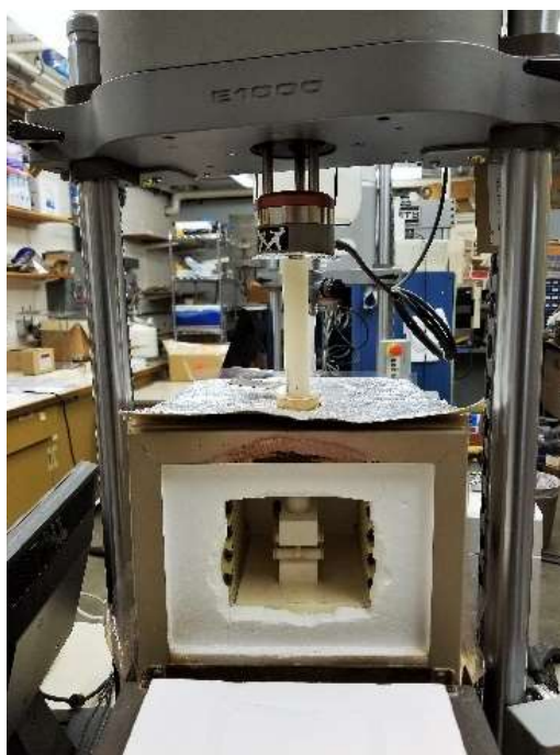
Figure 2.5: Image of the high temperature flexure setup placed inside the furnace. A Thermolyne 49700 series bench top furnace is placed within an Instron E1000 load frame.
