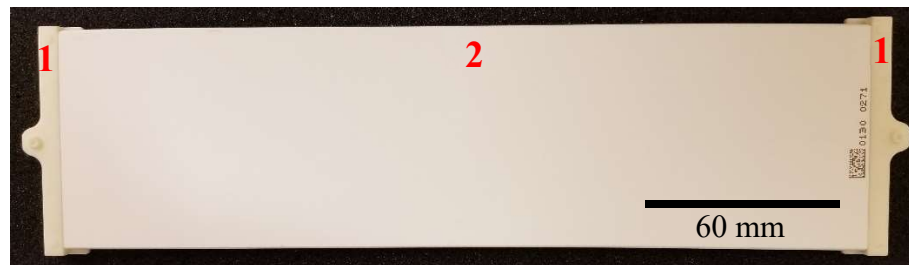
Figure 2.1: Picture of a complete single fuel cell. Areas marked with the number 1 are dense end caps and areas marked with the number 2 are porous tubes.
