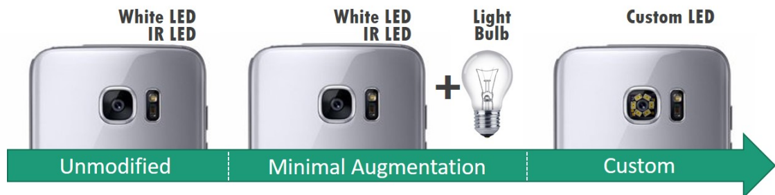
Figure 3.2: Three embodiments of HemaApp in increasing hardware augmentation.
