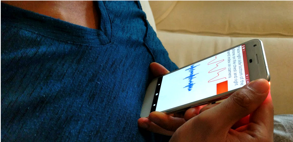
Figure 6.1: Measuring blood pressure using Seismo, a smartphone application that uses the built-in accelerometer and camera to calculate pulse transit time.
