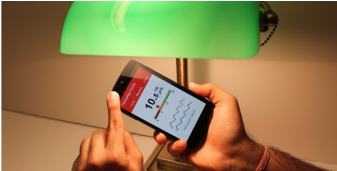
Figure 3.1: HemaApp is a smartphone application that noninvasively estimates blood hemoglobin concentration using a smartphone camera. Analysis of the color of the blood in a user's finger yields an estimate of the user's hemoglobin level. We evaluated the system using the smartphone's LED flash and incandescent light bulbs as illuminating sources.
