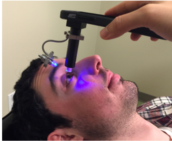
Figure 9.1: iPressure emulates fixed-force applanation tonometry using the hardware adapter pictured above. The clear acrylic cylinder is allowed to move freely within the black casing so that its mass provides a constant force on the patient's eye.
