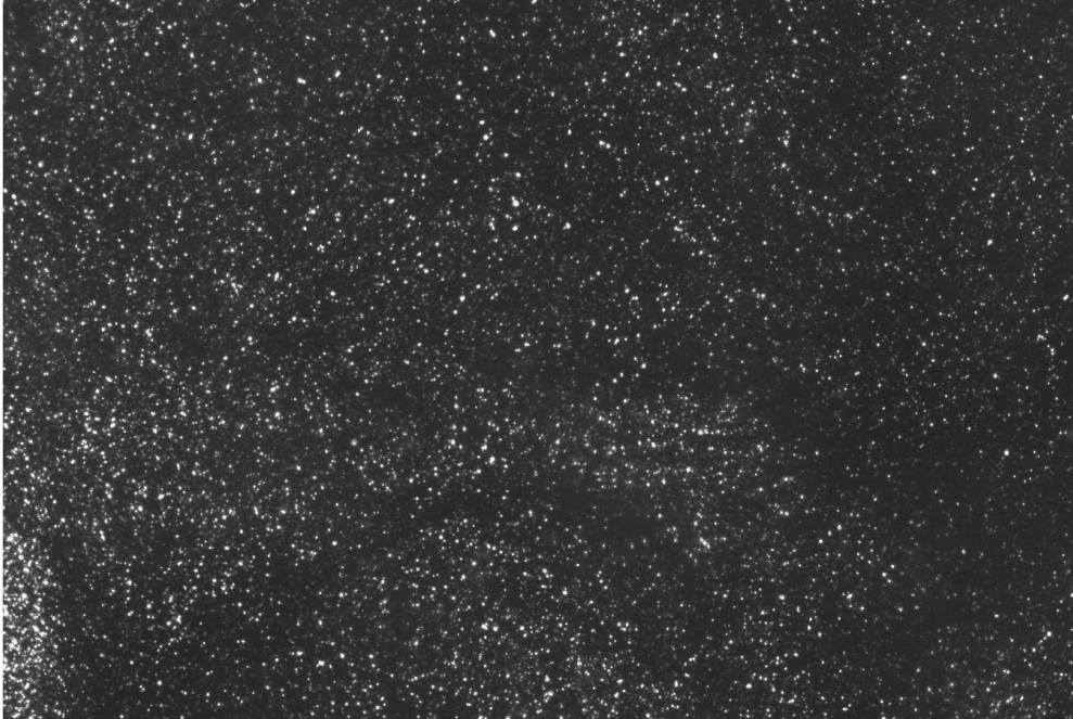
Figure 4.13: Sample particle image used to generate velocity fields in Dona (2015) 3
