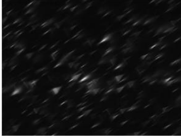
Figure 3.11: Astigmatism caused by refraction in air, acrylic and water 22
