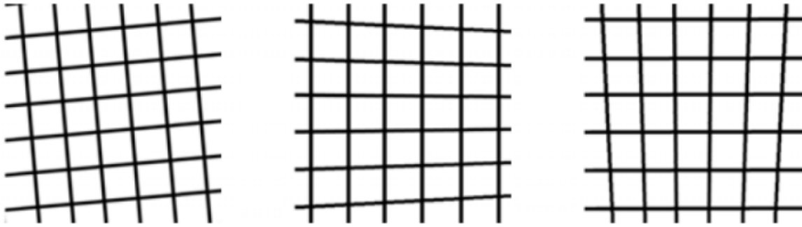
Figure 3.20: Distortion patterns from camera misalignment in each of the three rotational axes 22
