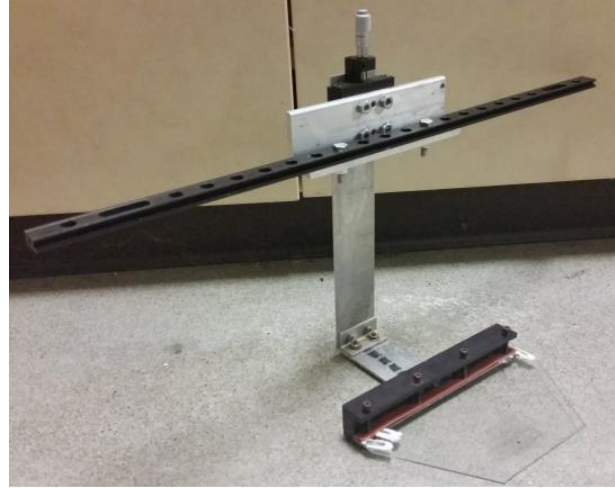
(b) Calibration rig with single-axis translation
