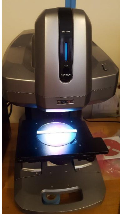
Keyence VR-3100. Non-contact 3D imager used for profilometry.
