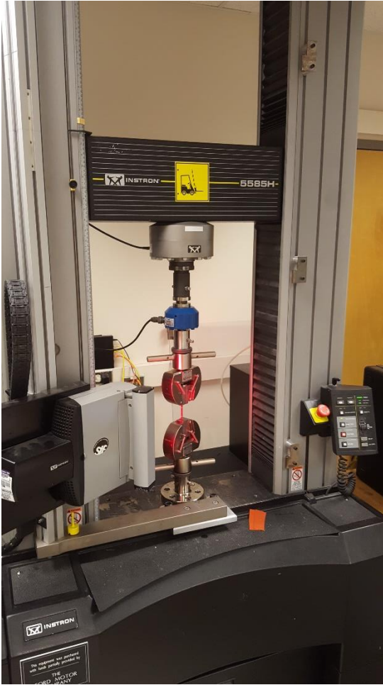
Instron load frame equipped with 50 kN load cell, 30 kN wedge grips, and an optical extensometer.
