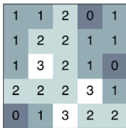
Figure 4.1: Example spike training binning of a 5 x 5 neuron array from Lee [20]. Each pixel displays the number of times the neuron spiked for a single bin. The color of each square is determined by the spike count at that (x, y) location, where brighter colors indicate higher spike rate.
