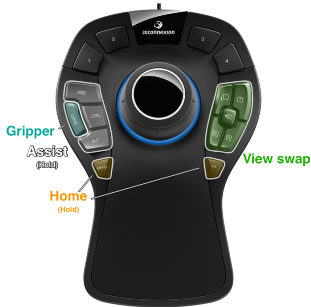
Figure B.1: The mapping of buttons to system controls used during the study.
