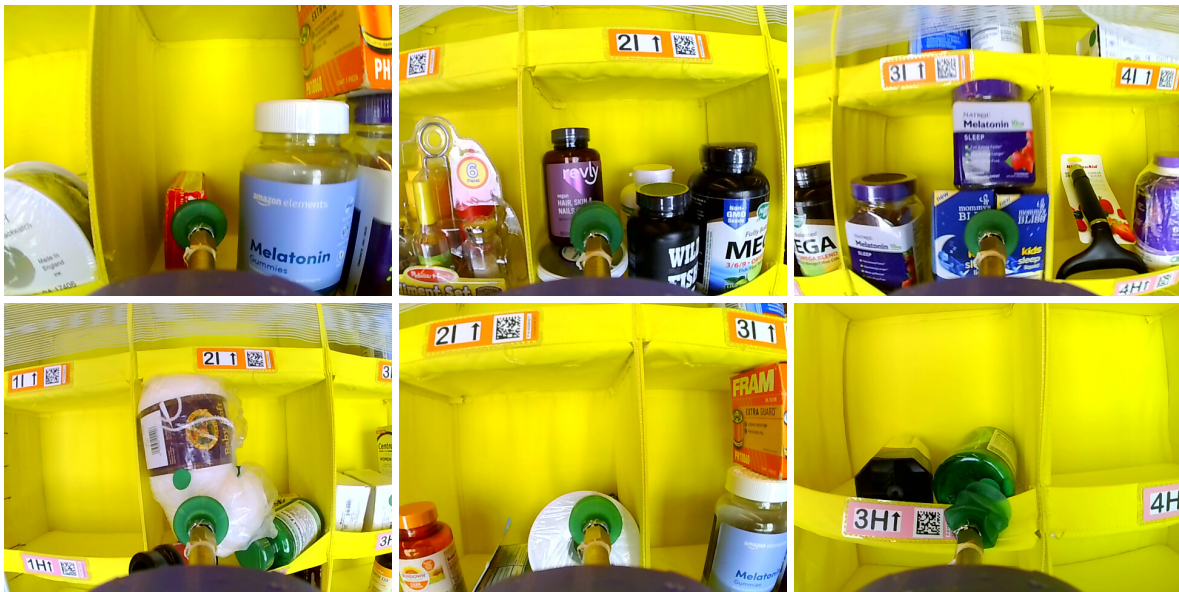
Figure 7.6: Still frames of failure cases during interaction in cluttered scenes. From top left, 1: a misaligned grasp pose (GP). 2: a misaligned grasp (GP) and the object shifting off the stack (MDF). 3: a poor grasp pose (GP) and suction being lost as the objects contact the lip of the shelf. 4: the robot hitting another object while extracting, causing it to fall from the shelf (MED). 5: the suction seal with the target object is lost due to the plastic wrapping on the object. 6: the robot halts (MOV) and a high force fault halts execution (NEW).
