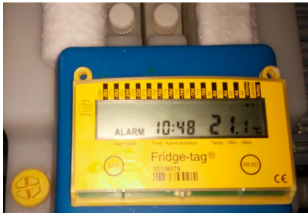
Figure 7.3: A 30 day temperature recorder (30DTR) in a Lao refrigerator showing two high alarms in the last two days
