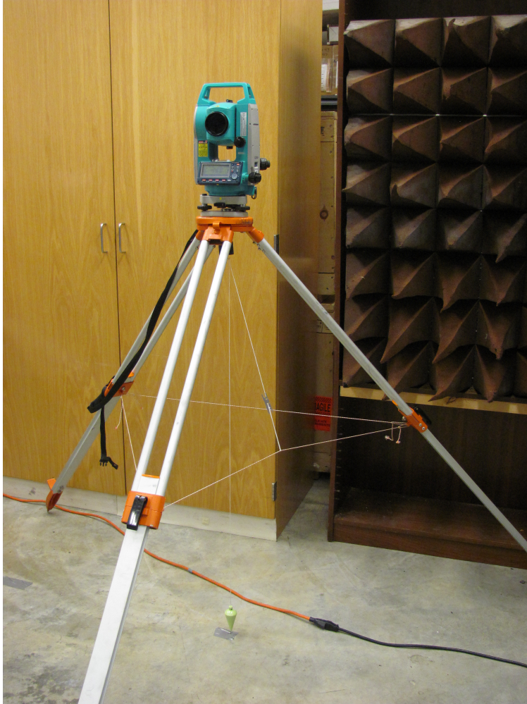
Figure B.2: Total station used to align the AUT
