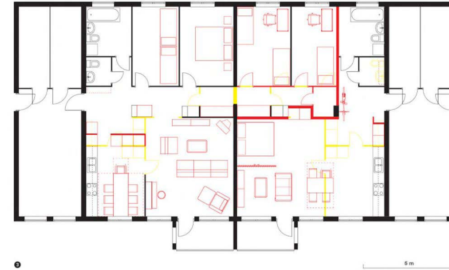
Figure 30: "An opening was made in the load-bearing wall separating two apartments to enable two bedrooms from one apartment to be incorporated into the other. The large apartment is 122 square meter and the smaller studio apartment is 56 square meters".
