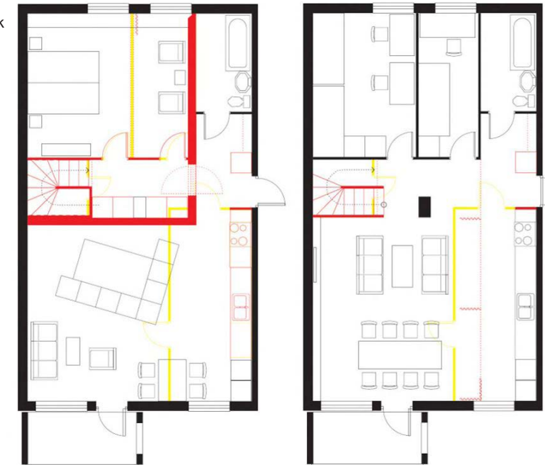
Figure 31: "Uppingegrad 30, The Duplex - explore the potential to link apartments vertically. An opening large enough for a standard stair was cut into the floor slab enough where a large closet had been".
