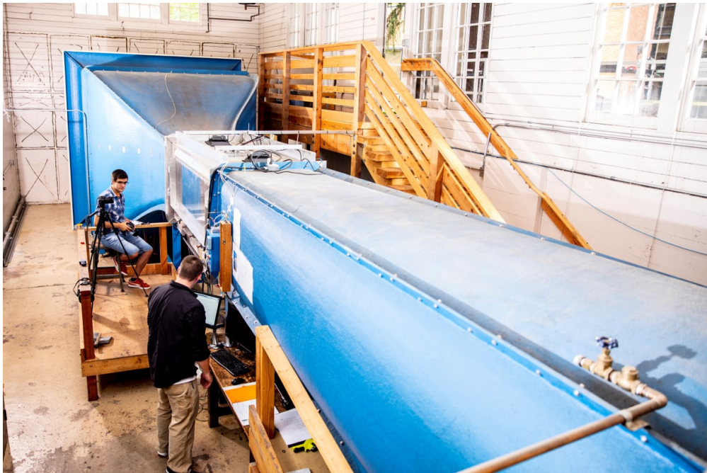
Figure 3.1: UW 3' x 3' low speed wind tunnel where experimental tests for this research were conducted. The clear test section can be seen in towards the back of the image.
