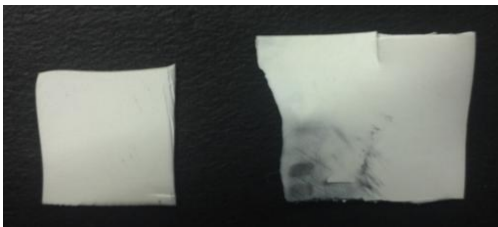
Figure 9.7: Samples with polished surfaces. The samples have final thicknesses of 1.10 mm on the left (Sample 1) and 0.65 mm on the right (Sample 2). The visible ink stains on Sample 2 are from porosity testing.
