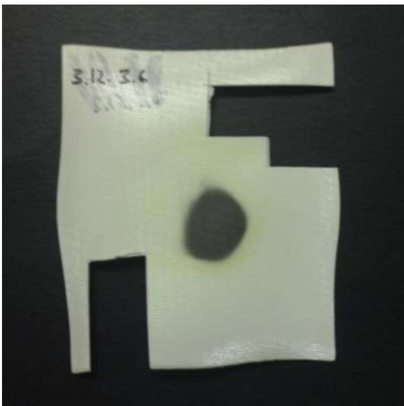
Figure 8.2: Sample foamed at 210°C. The dark circle in the middle is a translucent unfoamed section.
