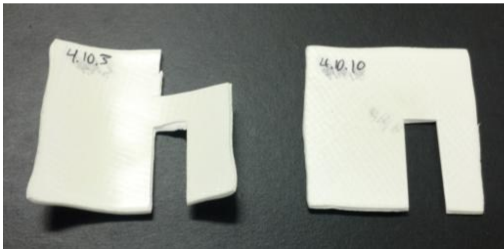
Figure 6.2: Samples foamed for 1.5 minutes (left) and 5 minutes (right). The curvature is apparent in the shorter foaming time sample. Rectangular cutouts are the result of taking samples for density measurement and electron microscopy.
