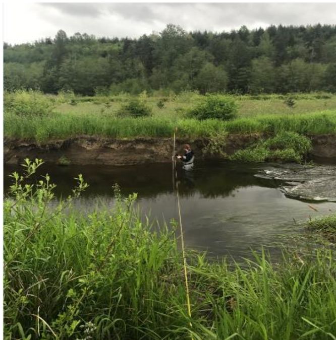
Figure 5. Select a cross-section site that is straight, has minimal upstream and downstream obstructions, and reasonably uniform bottom conditions.
