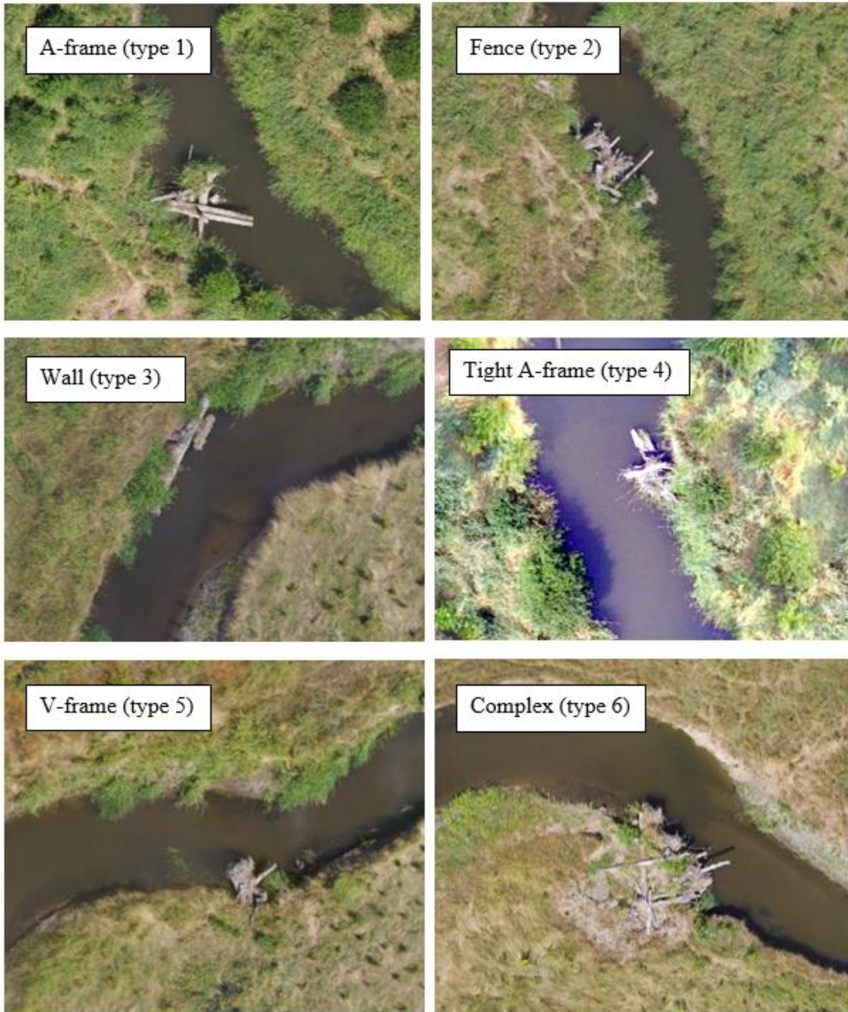
Figure 4. Six different LWM structure types identified in the Project reach. Flow direction for the first four images (types 1-4) is from top to bottom and from right to left for the latter two images (types 5 & 6).
