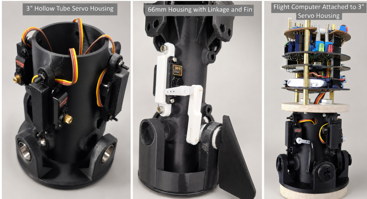
Figure 4: Steering-fin canister development hardware from multiple views, with background edited away. Left: 3-inch hollow tube servo housing. Center: 66 mm housing with servo linkage and fin. Right: V2 flight computer attached to the 3-inch servo housing..
