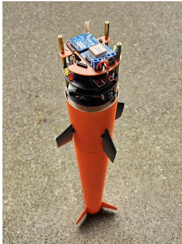
Figure 5: V2 modified Apogee Mako rocket with flight computer installed, nose cone removed.
