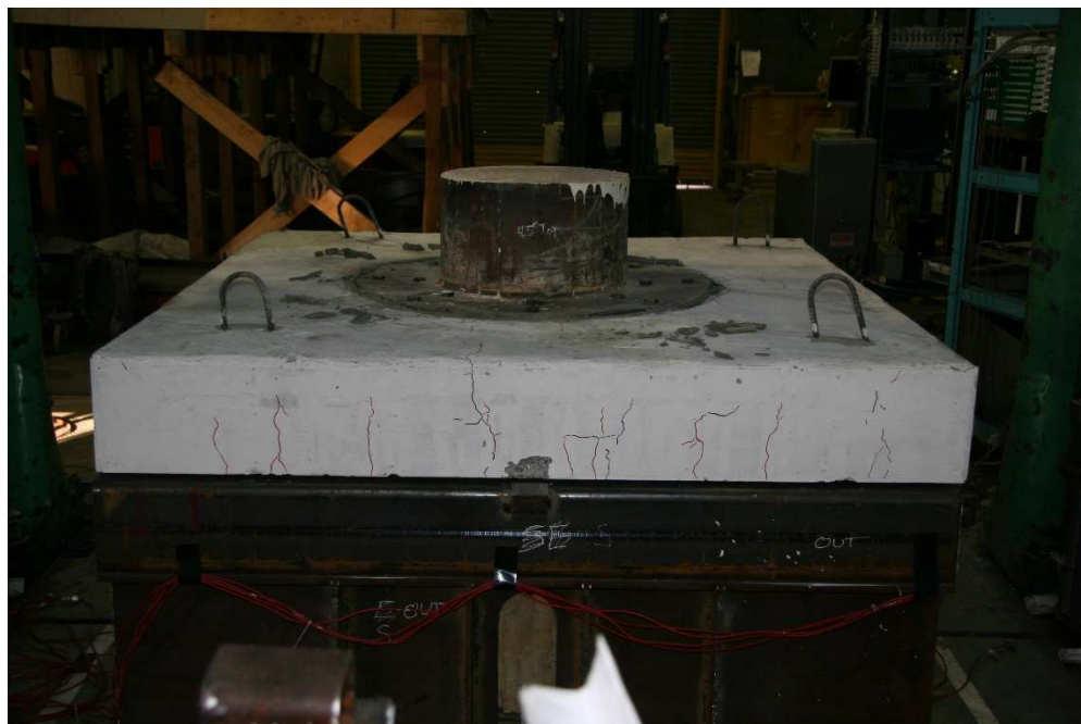
Figure 6.38. Cracking South Face – Load Removed (PTB_9_2_0_P)
