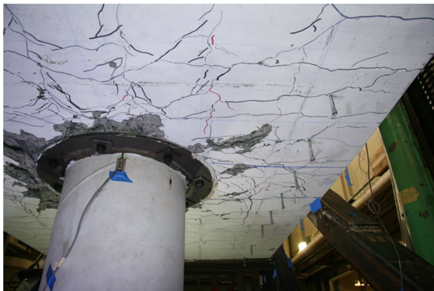
Figure 4.27. Damage on North Side of Bottom Face – 6.35% Drift (PTB_4.5_1_0_6)
