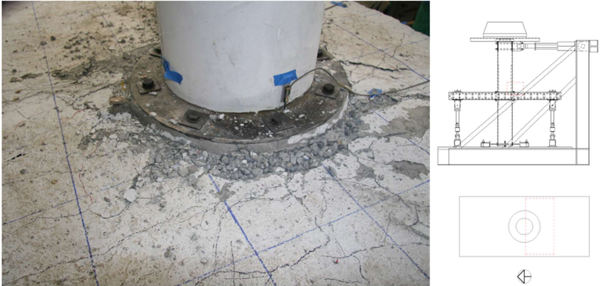
Figure 4.26. Damage on South Side of Top Face – 6.35% Drift (PTB_4.5_1_0_6)
