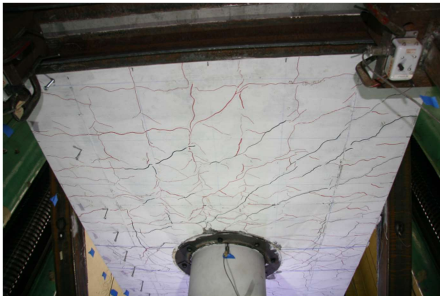
Figure 4.18. Spalling on South Side of Bottom Face – 4.11% Drift (PTB_4.5_1_0_6)
