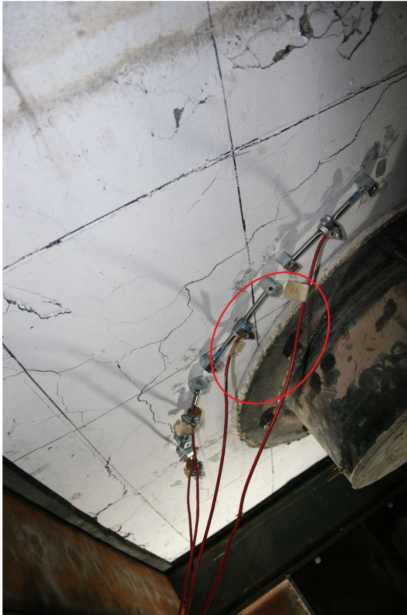
Figure 6.12. Deformation of Concrete around Ring Flange on Bottom Face – Post Test (PTB_4.5_1_0_P)
