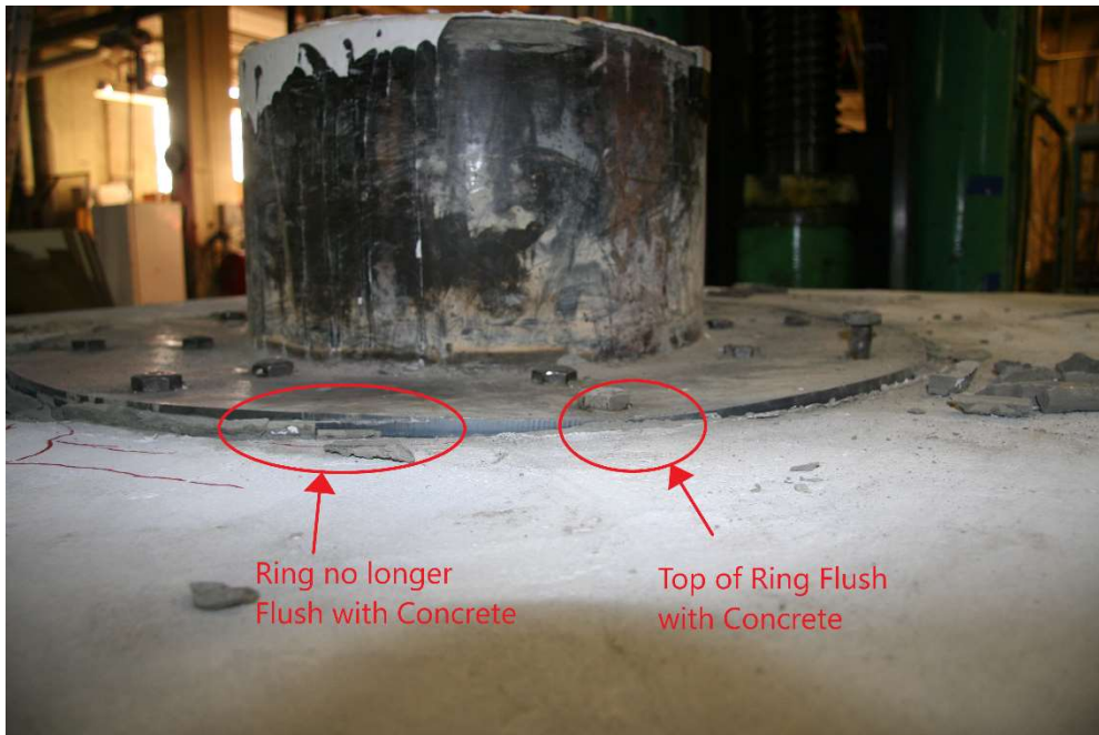
Figure 6.40. Warping of Top Ring Flange – Load Removed (PTB_9_2_0_P)
