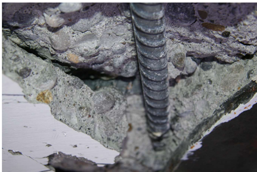
Figure 4.28. Exposed Bar on North Side of Bottom Face – 6.35% Drift (PTB_4.5_1_0_6)
