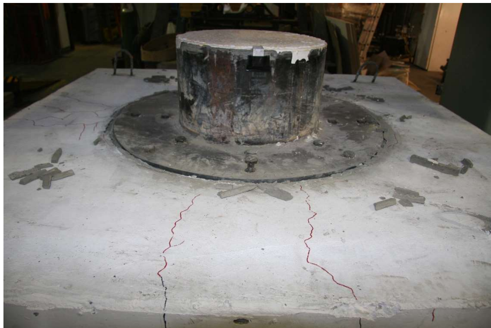
Figure 6.37. Cracking North Side of Top Face – Load Removed (PTB_9_2_0_P)
