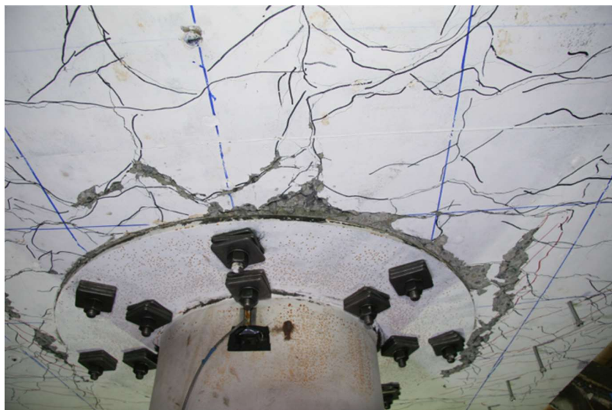
Figure 4.44. Spalling on North Side of Bottom Face– 5.00% Drift (PTB_9_2_0_6)
