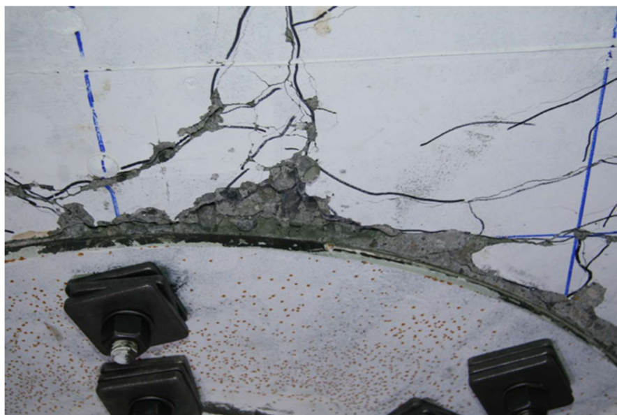
Figure 4.45. Crushing on North Side of Bottom Face– 5.00% Drift (PTB_9_2_0_6)
