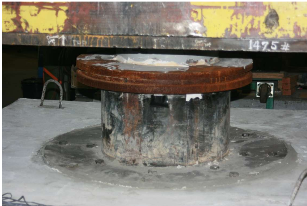
Figure 6.28. Deformation of Top Ring Flange – 600 kips Post Peak (PTB_9_2_0_P)
