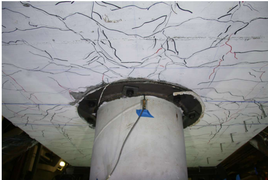
Figure 4.17. Spalling on North Side of Bottom Face – 4.11% Drift (PTB_4.5_1_0_6)
