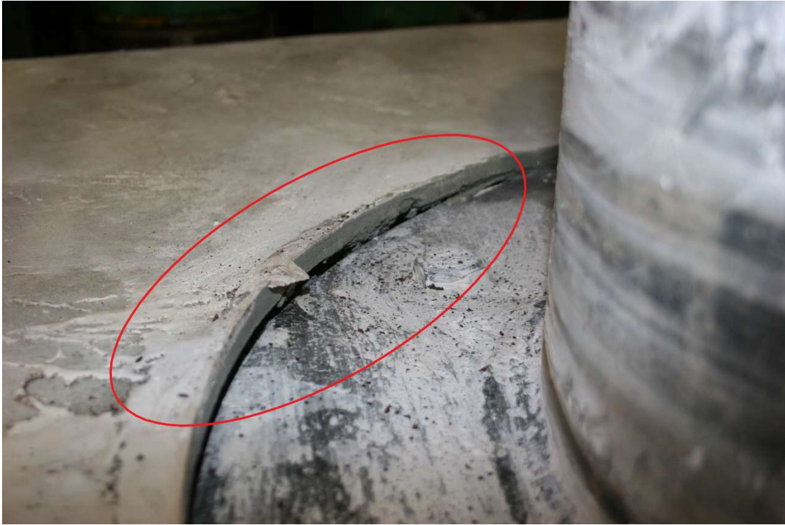
Figure 6.11. Deformation at Ring Edge of Top Column – Post Test (PTB_4.5_1_0_P)
