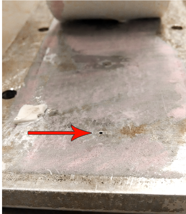
Figure 6.3: The holes go all the way through the aluminum plates and connect to the compression fittings on the other side.
