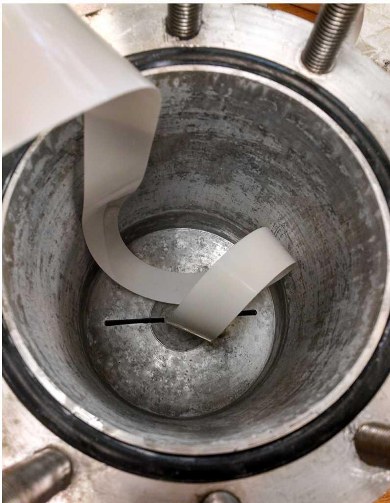
Figure 4.5: View into the vessel showing the slit on the bottom through which the polymer can enter and exit the pressure vessel.
