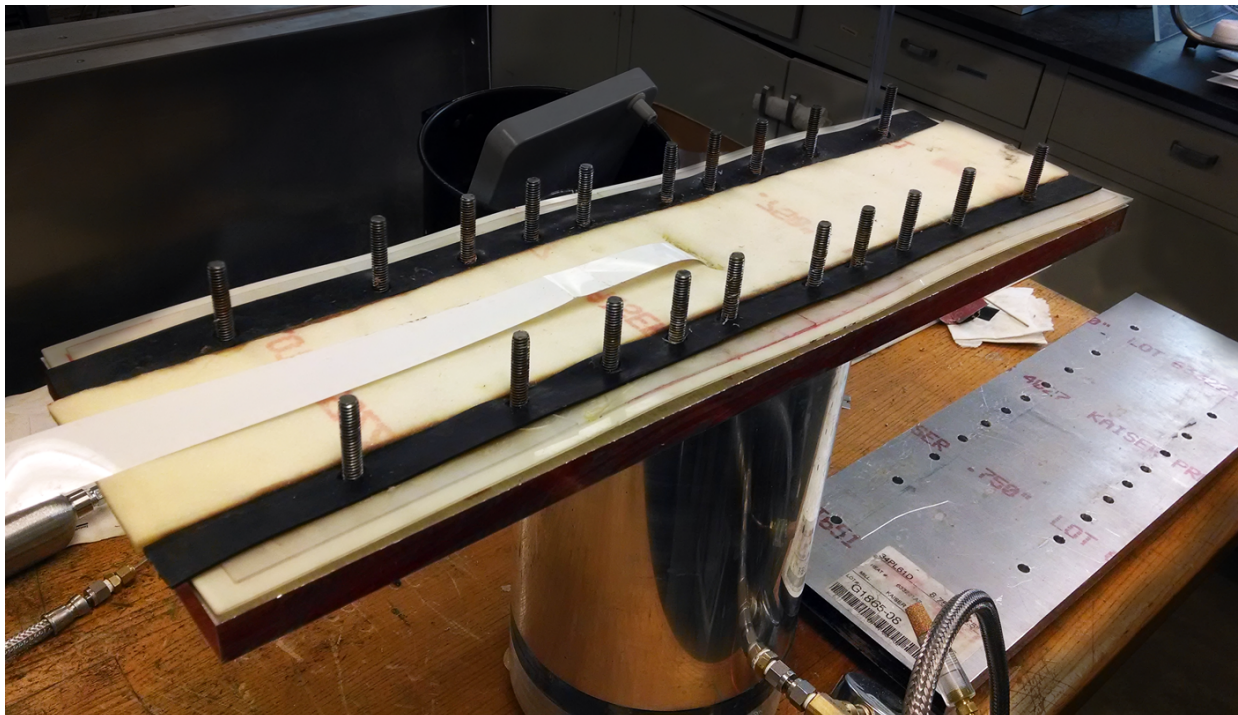
Figure 5.1: View of the bottom half of an example seal setup. The porous material (white) is the working seal, while the black rubber (neoprene) serves to block flow transversely.
