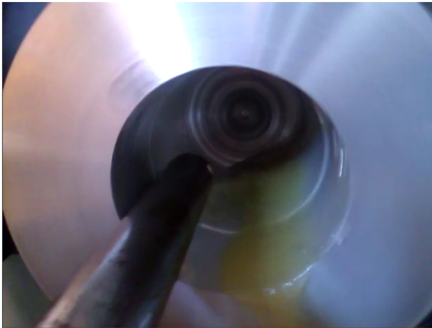
Figure 4.11: Inside view during the boring operation. The passes are very small (approximately 0.015") and the rotation speeds less than 80 RPM on average. The liquid seen is lubricant/coolant which also helps wash away the chips.
