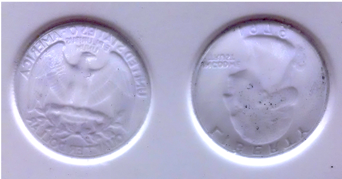
Figure 5.18: A US quarter was pressed into a PET microcellular sheet from MicroGREEN™ using a vise. The detail is permanently imprinted on the sheet.
