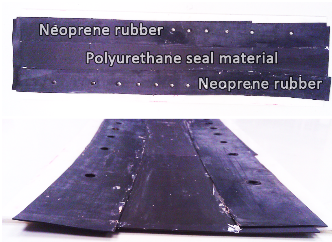
Figure 5.3: Seal material setup. The material used is 1/32 inch 20 lb/ft 3 polyurethane open-celled foam. Along the sides, 1.5 inch strips of 1/32 inch thick neoprene rubber are attached for sealing the flow transversely.
