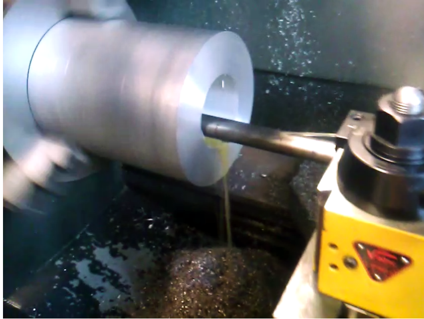
Figure 4.10: Vessel boring setup on the HAAS TL-3 CNC lathe.
