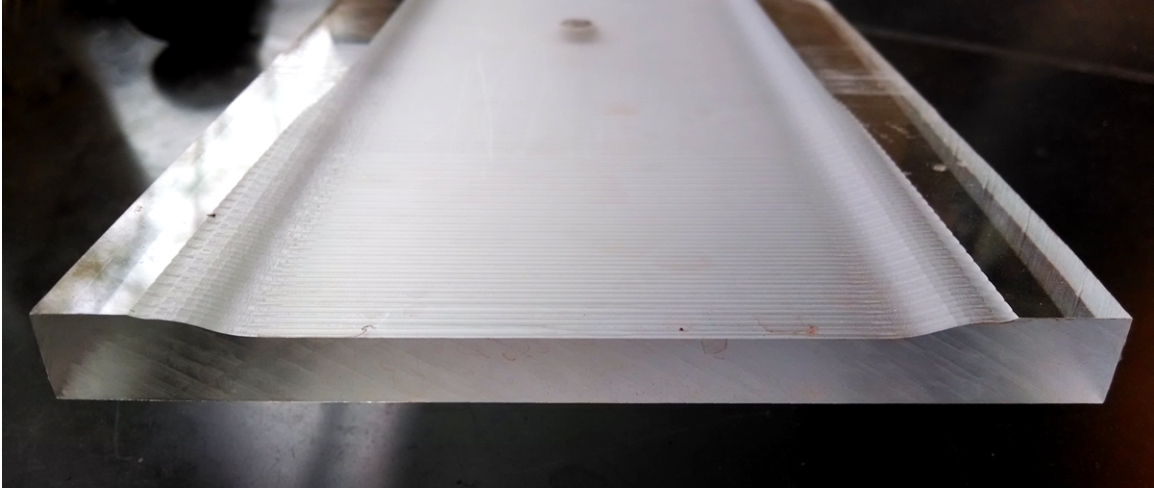
Figure 5.9: Curvature machined in the polycarbonate plate to clamp the seal material edges.
