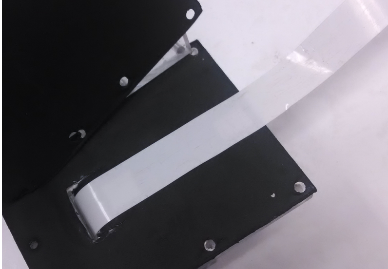
Figure 2.2: A dynamic seal design where the film is clamped by two soft (foam) materials that provide the seal. The film enters the pressure vessel below (not seen) through the slit.
