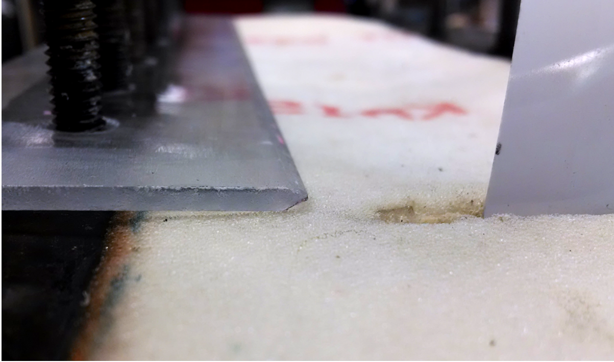
Figure 5.6: Photo of the polycarbonate V-shaped piece used as a barrier for transverse flow. Since the edge does not have infinite curvature as does a rectangle corner, it was hypothesized that the seal material would conform to the shape and not produce any gaps.
