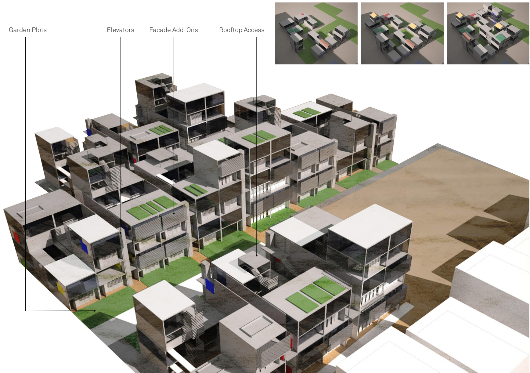
Fig 6.6 Rendering showing one quadrant's fully formed development with varying heights as buildings get added on over time.
