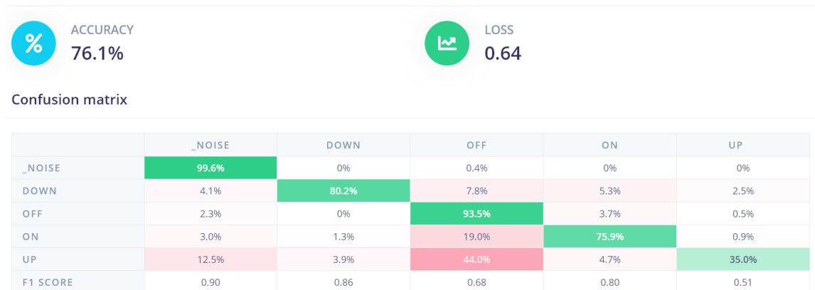
Figure 37. Confusion matrix of trained the reduced CNN by using 32-channel vocoded speech.
