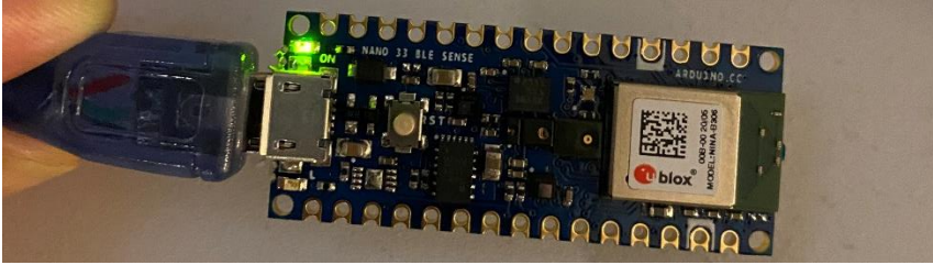
Figure 40. LED light (orange) does not blink when the confidence score in the corresponding category does not meet the requirement.
