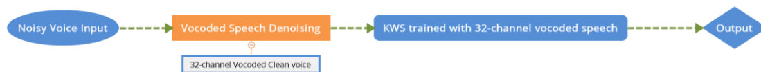
Figure 27. Using Vocoded Speech Denoising system to convert noisy voice input into 32-channel vocoded clean voice, then feed clean voice into the KWS trained with 32-channel vocoded speech.
