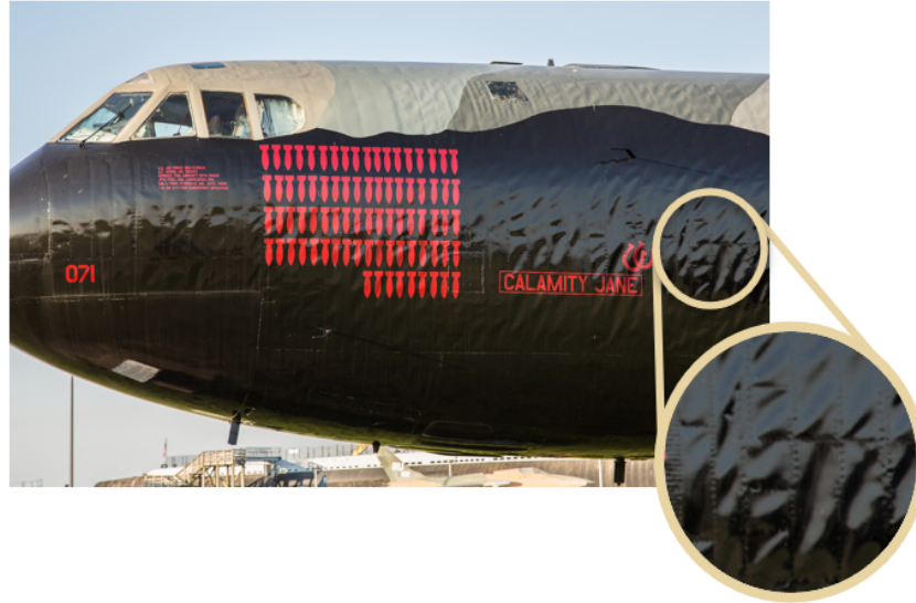
Fig. 3 Effects of aerodynamic loads on constrained skin panels
