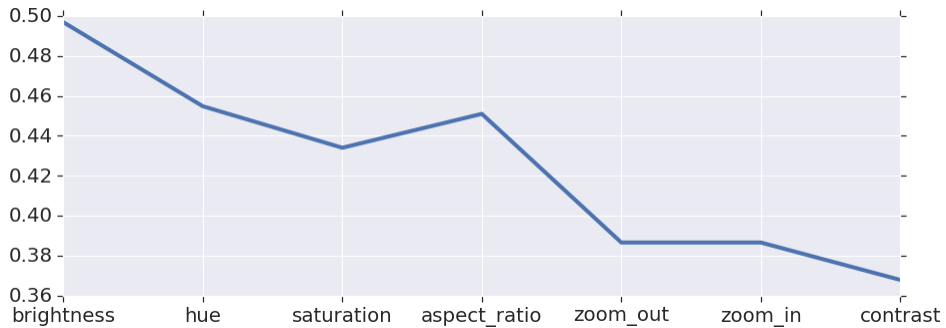
(b) Relative importance of the first block of ResNet-18 for predicting each of the data augmentation ranking tasks.
