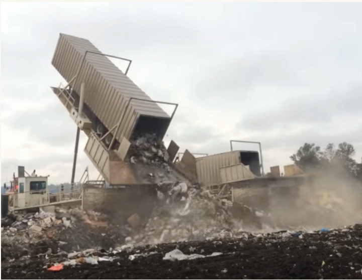
Fig. 41 A 'tipper' at the CHRLF empties waste into an open cell. Photo: King County
