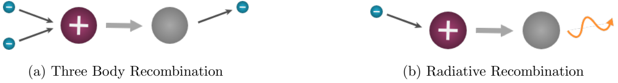
Figure 4.2: Recombination processes. Three body recombination (a) is the reverse process for electron impact ionization where two electrons hit a positively charged ion. One of the electrons gets bound and the other electron absorbs the extra energy. On the other side, an electron gets absorbed by a positively charged ion and the excess energy is released as a photon (b).
