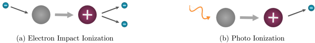
Figure 4.1: Ionization processes. In highly collisional plasmas where electron mean-free-path is short the main cause of ionization is electron impact ionization shown in (a), where a high energy electron hits a neutral atom and kicks the last electron out of its orbit. On the other hand, if plasma is opaque and radiation is well trapped a neutral atom absorbs a photon and the excited electron leaves its orbit leaving a positively charged ion (b).
