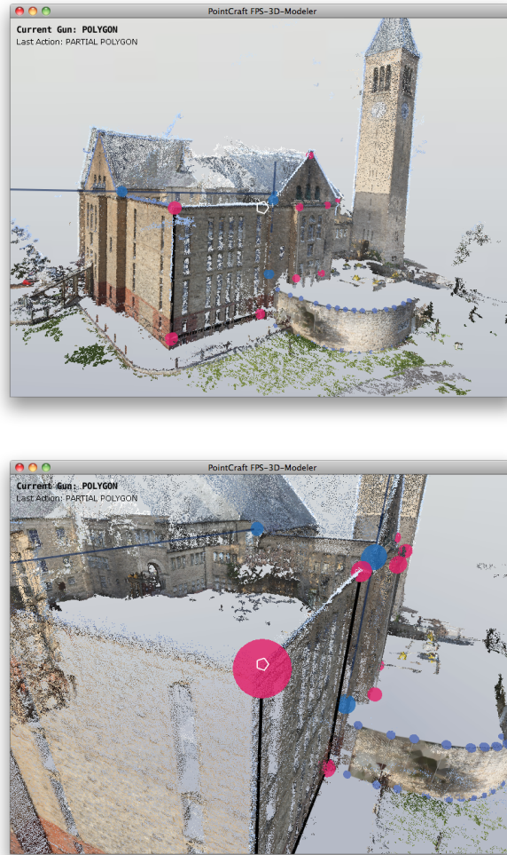
Figure 5.3: Two screenshots of the PointCraft user interface showing a user defining a polygon.
