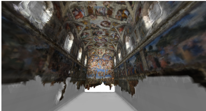
Figure 5.12: The result of running automatic Poisson Surface Reconstruction on a point cloud of the Sistine Chapel augmented with points sampled from wall and floor geometry added using PointCraft.
