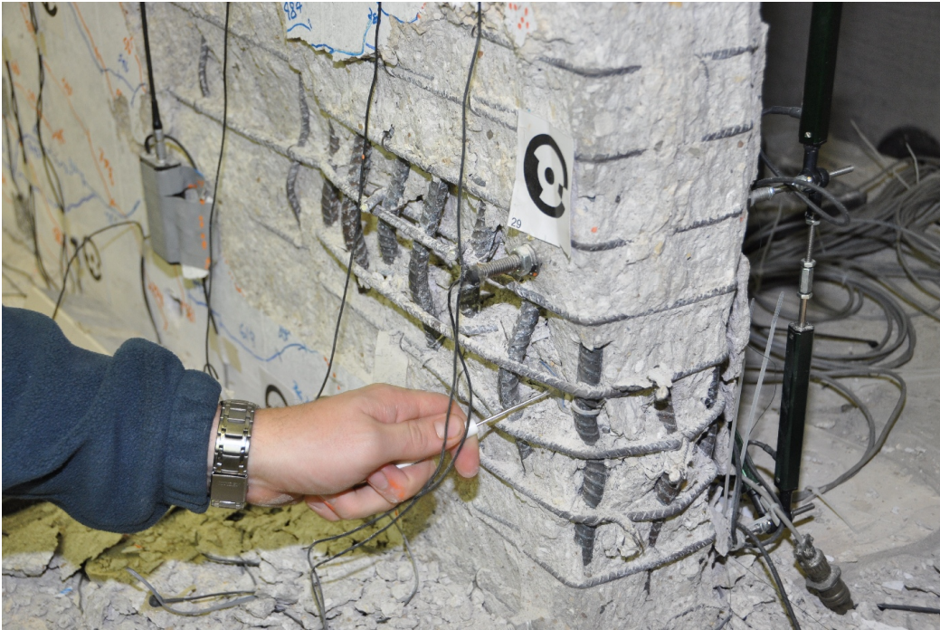
Figure 4.33: Front corner of EWP at E+ peak (2.25% D.C. (A), Step 955)
