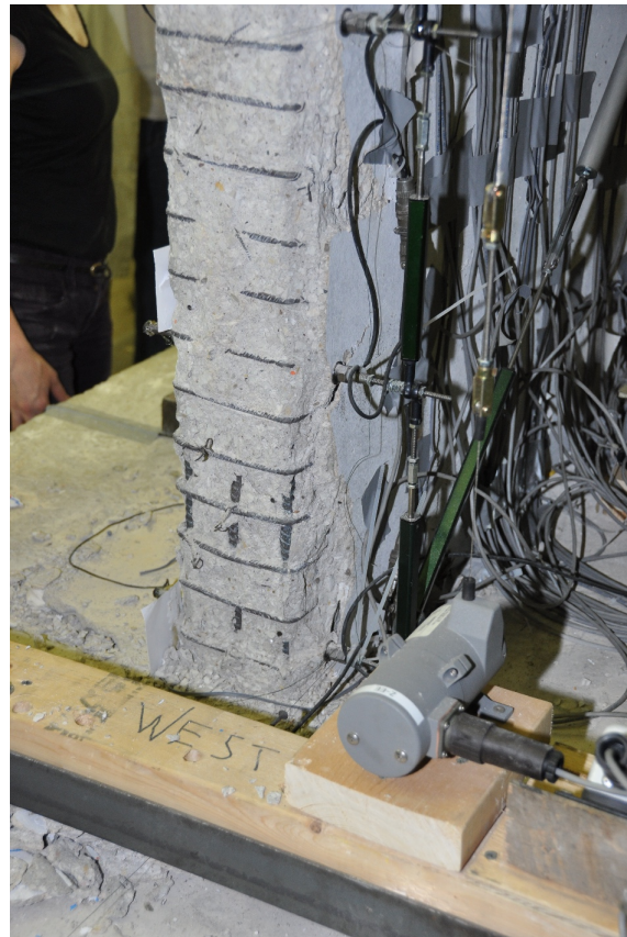
Figure 4.31: Backside of EWP at 2.20% (2.25% D.C. (A), Step 954)
