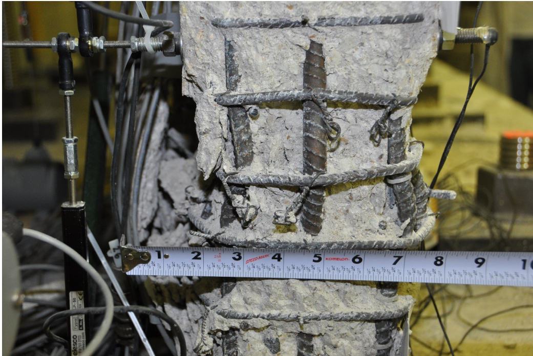
Figure 4.39: West facing edge of WWP at W- peak (2.25% D.C. (A), Step 1003)
