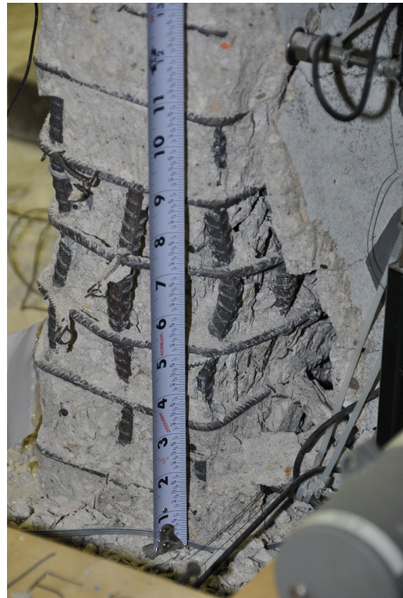
Figure 4.36: Backside of EWP at E+ peak (2.25% D.C. (A), Step 955)
