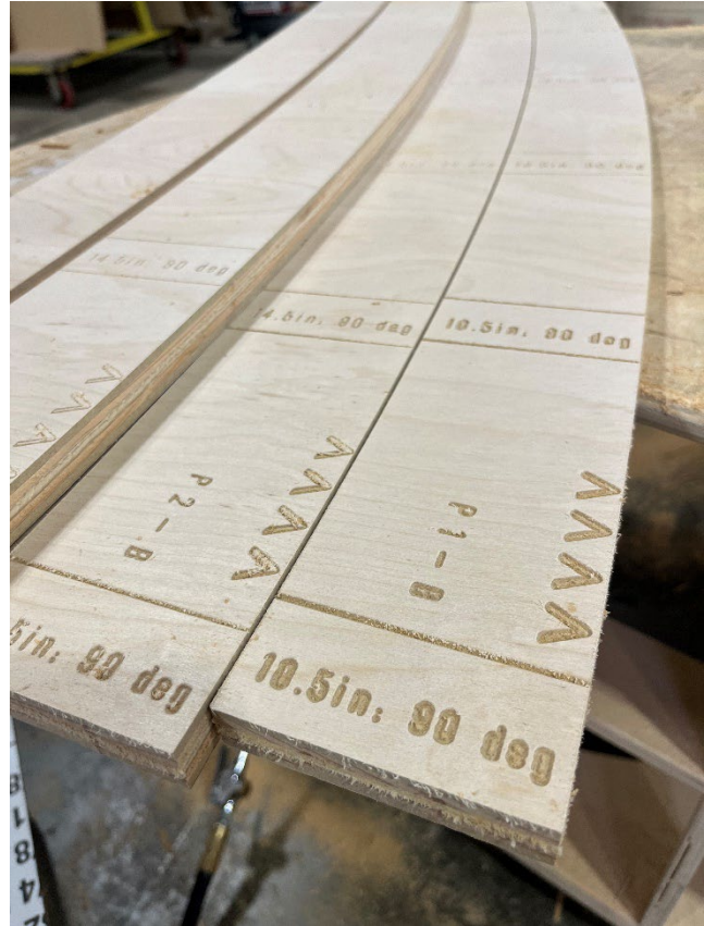
Figure 17: This labeling system represents an approach that will be further investigated by Turner Construction as a way to encode fabrication information into the CNC'd parts, as opposed to the assembly information encoded into the parts used in the assembly trials.
