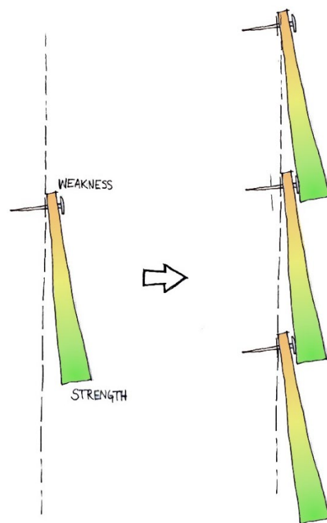
Figure 25: The overlap of strengths and weaknesses can be likened to shingle siding. A lone shingle is a weak weather protection barrier, but by overlapping them to function as parts of a larger system they become effective.
