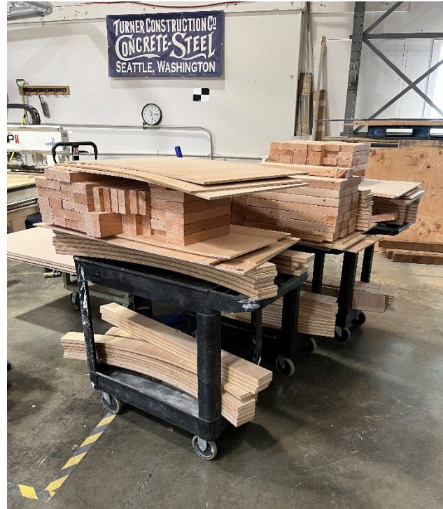
Figure 11: Parts for each wall kit organized onto rolling carts.
