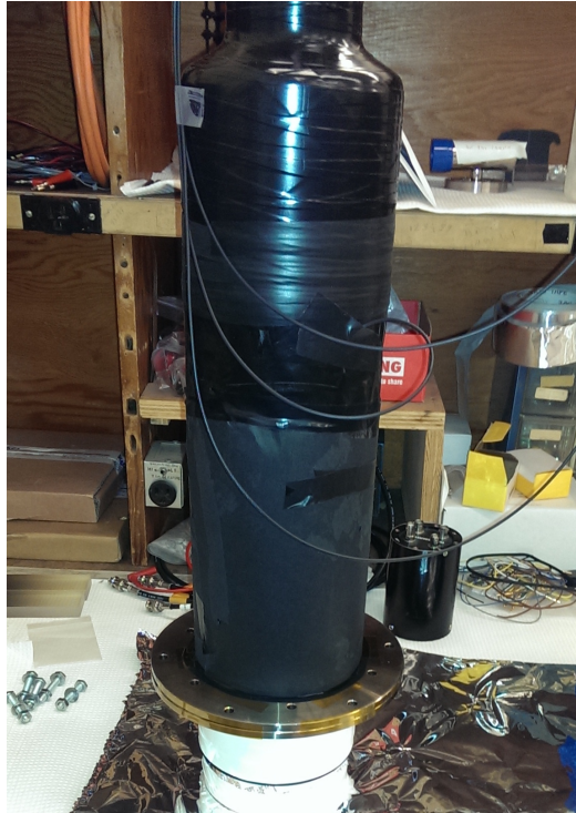
Figure 3.5: Photo of the scintillator, light guide and PMT with wrappings.
