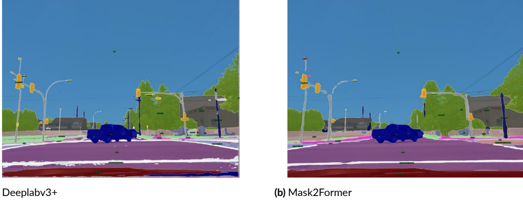
Figure 4.2: Domain models fail confidently for certain infrastructure classes like manhole . Even though SAM has correctly generated mask for two manholes in the SLI as in Figure 3.11, domain models fail to classify any pixels in the region as class manhole through MC runs. In this case, the both Deeplabv3+ (panel a) and Mask2Former (panel b) “confidently” predicted the mask wrongly as road . This is a potential limiting factor for the iterative sampling pipeline proposed in Chapter 3.
