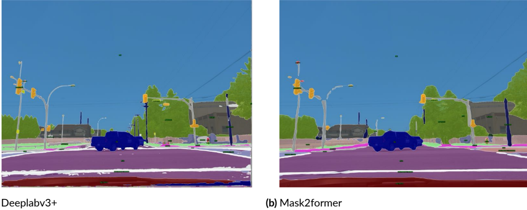
Figure 1.2: Domain models prioritize different aspects of semantic segmentation quality: (a) Deeplabv3+ extracts better boundaries for objects while (b) Mask2former produce more coherent masks. They agree on most objects in the scene but disagree on road infrastructure elements, e.g., guardrail, pole, etc. This is a major limitation preventing them from being applied to automated safety assessment.
