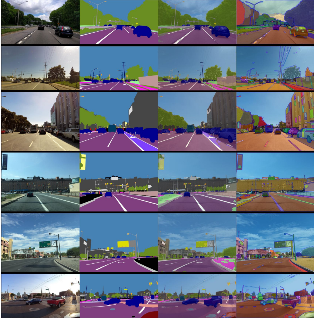
Figure 1.3: Examples of domain segmentation model (Deeplabv3+) vs. SAM. The four columns from left to right are (a) original SLIs, (b) ground truth labels, (c) domain model results, and (d) SAM results. Notice SAM masks are of high quality even though it has not seen this dataset in its training. The domain model has seen these data during training.
