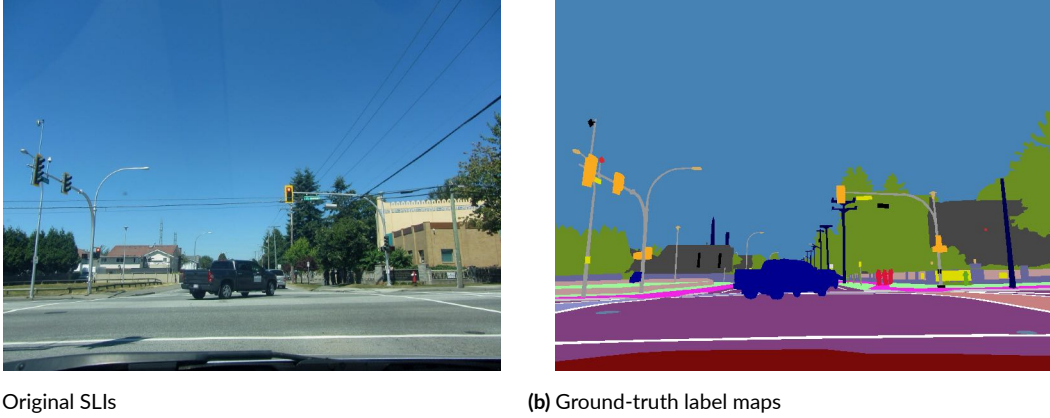
Figure 2.1: Mapillary Vistas dataset include (a) high-quality SLIs and (b) their ground truth segmentation map labels. These ground truths (panel b) demonstrate pixel-wise segmentation annotation with precise object boundaries. The annotation exhibits sophisticated class differentiation between closely related roadway elements, e.g., traffic signals, poles, and utility poles, that are coarsely treated in other datasets. This dataset has a comprehensive coverage of both dominant classes like cars and roads, plus safety-relevant minority classes, e.g., traffic signals, curbs, guard rails, fences, etc.
