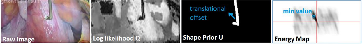
Figure 2.8: The optimal offset for U in order for it to align with Q is the vector from the image center of the energy map to the min valued point in the energy map.
