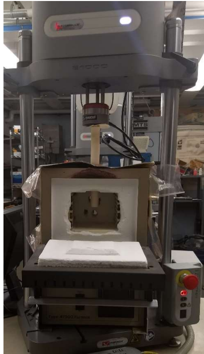
Figure 2.9: Instron E-1000 UTM loaded with Thermolyne 47900 bench top furnace used for flexural tests.
