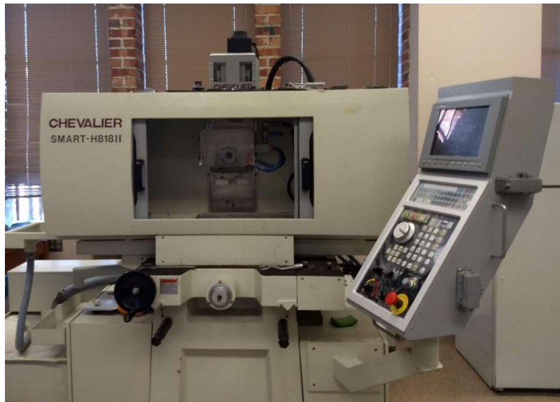
Figure 2.3: Chevalier Smart-H818II surface grinder used for the sample preparation
