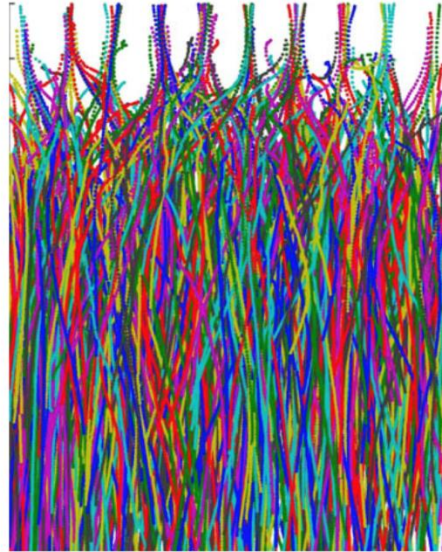
Figure 5.6. Long particle tracks obtained using 3D implementation of the ICCRM algorithm. 191
